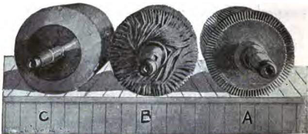
FIG. 130.—TOOTHED-CORE ARMATURE IN VARIOUS STAGES OF CONSTRUCTION.
